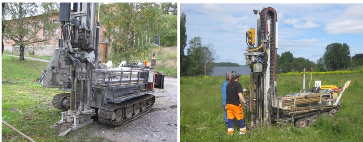
Figur 7-3. ODEX-borrning i deponi (Serti, 2010, 2012).
