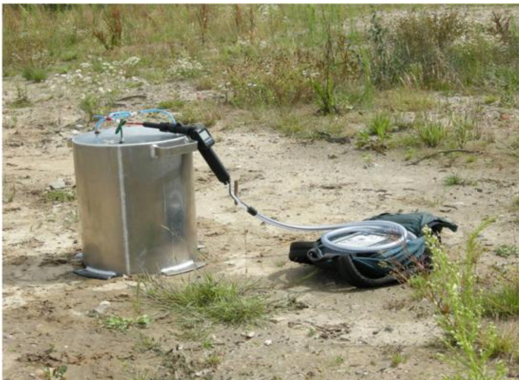
Figur 6-8. Öppen statisk kammare (University of Hamburg, Institute of Soil Science, Project MiMethox).
